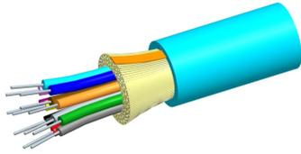
Fiber indoor cable, Low Smoke Zero Halogen Distribution, 6 fiber single-unit, Multimode OM3, Meters jacket marking, Aqua jacket color
